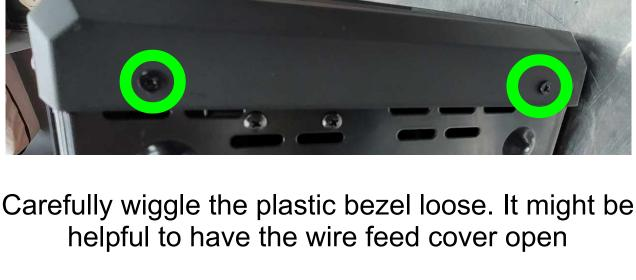
to access The two wires connected to the LCD circuit board
