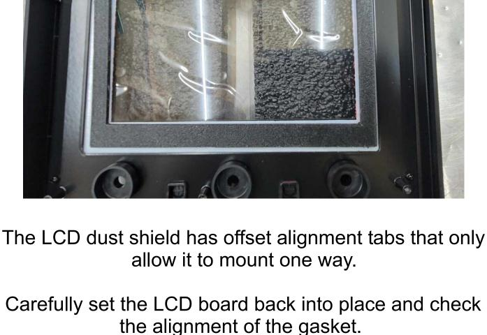
Reverse these steps for reassembly. Be careful not to over tighten the LCD board screws.
